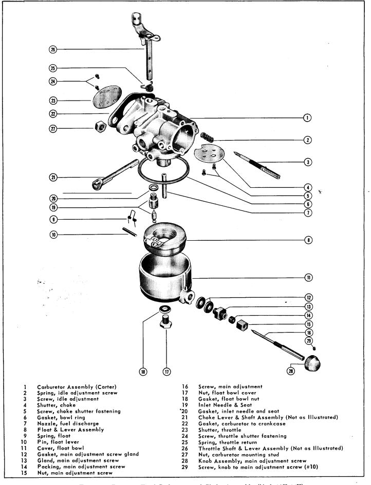
Figure 7. Pressure Feed Carburetor and Choke Assembly (Mark 20H-55H)
